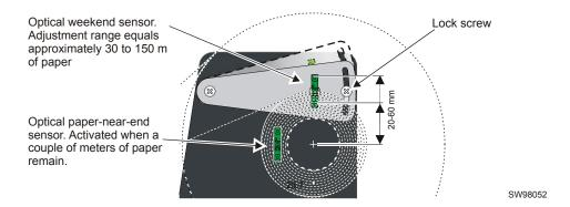
The paper-near-end sensor alerts the system when a couple of meters of paper remain on the roll. The purpose of this sensor is to get an early alert so that you can replace the paper roll in time in remotely located kiosks.
